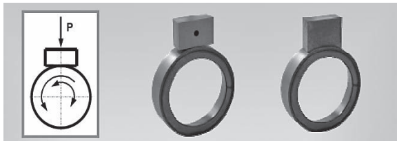
Figure 1 Illustration of tribosystem
