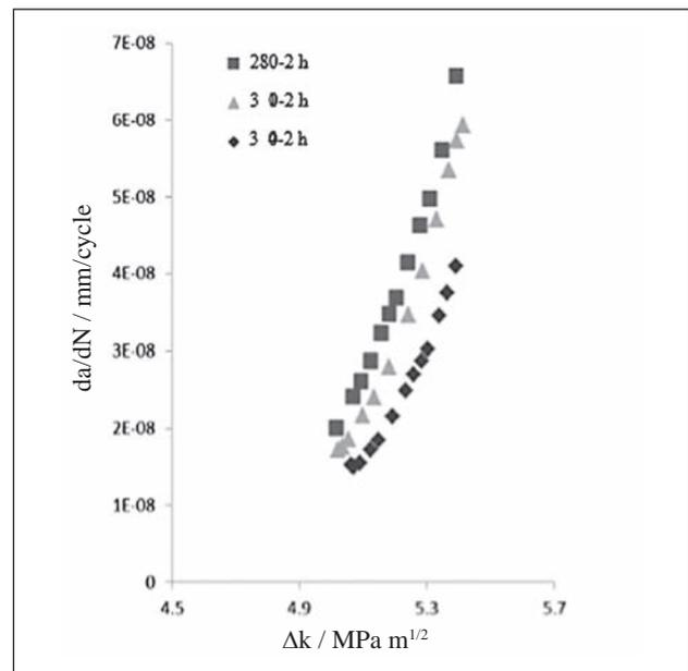
**Figure 3** The fatigue crack propagation ( $da/dN$ ) and stress intensity ( $\Delta k$ ) of nodular cast iron in various temperatures holding time of 120 minutes
