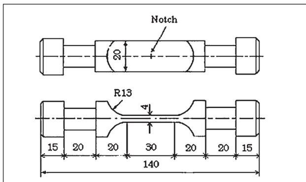
**Figure 1** The specimen of the fatigue crack test [12]
