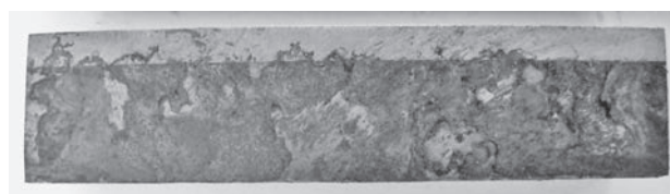
Figure 2 Condition of the sample after 48-hour exposure in salt chamber
