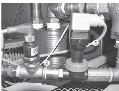
Figure 9 Location of converters for measurements of flow-rate 1 and pressure 2
