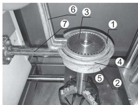
Figure 10 CDFIH system. 1 – MF inductor, 2 – HF inductor 3 – gear wheel, 4 – sprayer, 5 – cylinder, 6 – MF bus-bars, 7 – HF bus-bars
