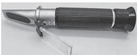
Figure 8 The meter for the concentration of the quenchant
