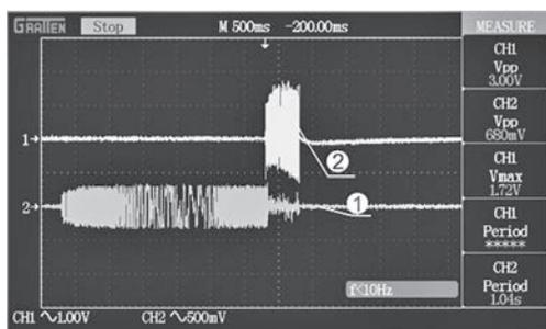
Figure 7 Oscillograms of MF current (1) and HF current (2)
