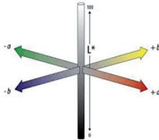
Figure 1. Graphical presentation of CIE L*a*b* colour space where: L* - lightness of the colour and takes the values from 0 (absolute black) to 100 (absolute white) and lays in the plain normal to axes a* and b*; a* - determine the position of colour on green- red axe taking the values from - 80 (absolute green) to + 80 (absolute red); b* determine the position of colour on blue – yellow axe taking the values of - 80 (absolute blue) to + 80 (absolute yellow).
