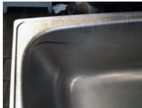
Figure 3. Damaged bath tube with wrong lubrication and high blank holder force
