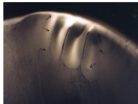
Figure 4. Damaged bath tube without using of bead
