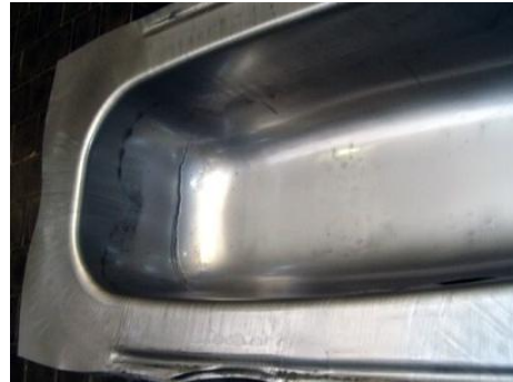
Figure 2. Damaged bath tube at high blank force
