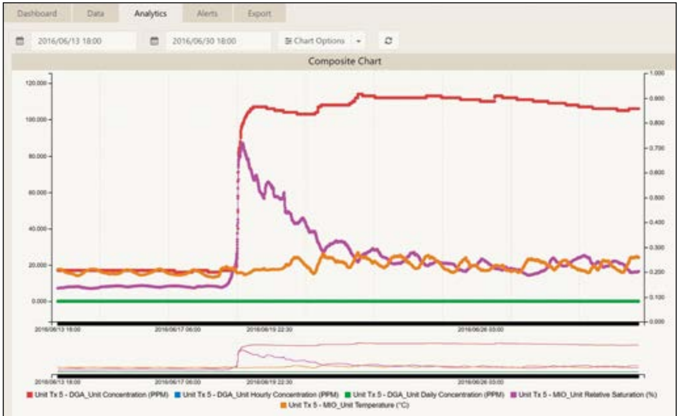
Composite data: DGA, relative humidity and oil temperature
