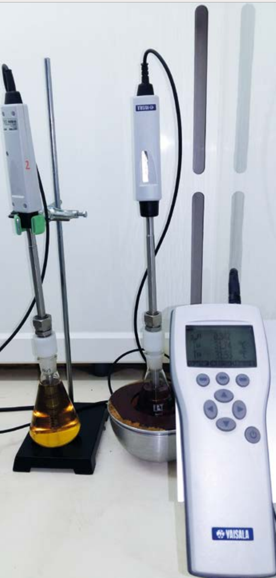
Figure 8. Apparatus for the measurement of the relative humidity and temperature
