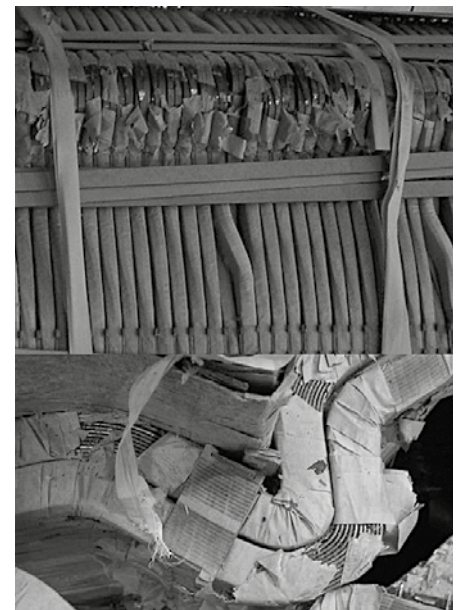
Figure 4. Photograph of windings that underwent deformation [9]
