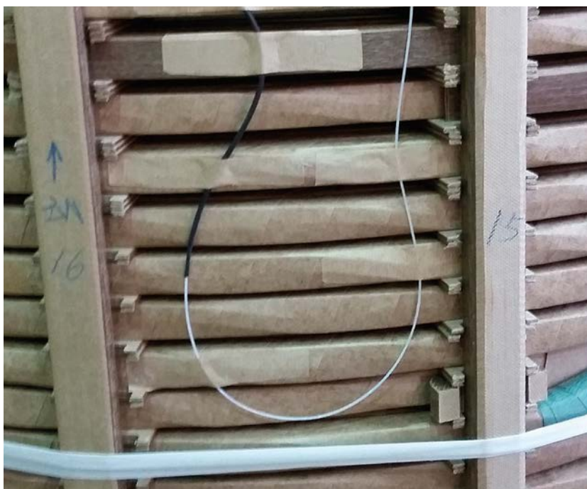
Figure 8. The press wood spacer is inserted between the winding turns. The coupled sensing fiber picks up vibration signature.
