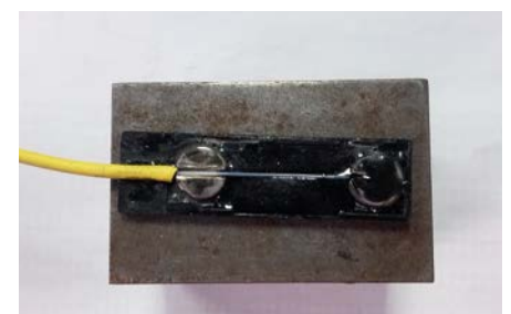
Figure 7. Example of internal structure of the VibroFibre with emphasis on the fiber optics
