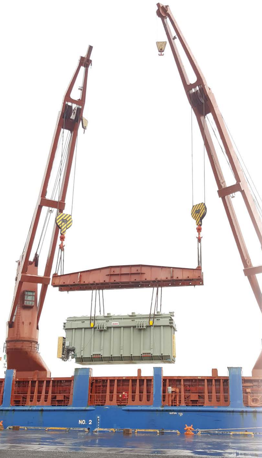
Figure 3. Transformer being off-loaded from the ship onto the barge
