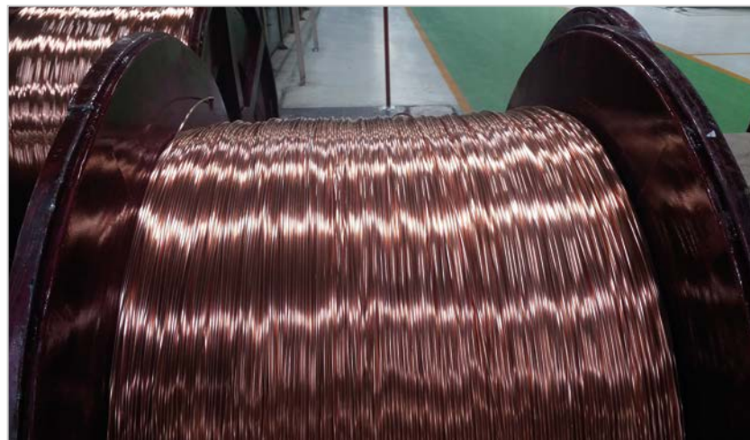
Figure 4. Drawn copper wire after the wire drawing stage
