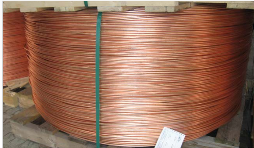
Figure 3. An 8-mm-diameter copper wire rod
