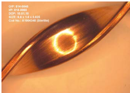
Figure 20. A flawless Cu-strip after the torsion test
