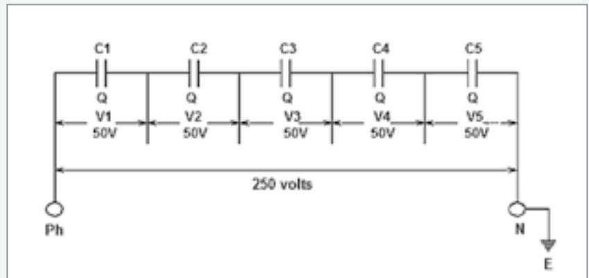
Figure 1. A specimen circuit of capacitors, each of 20 nF, connected in series
