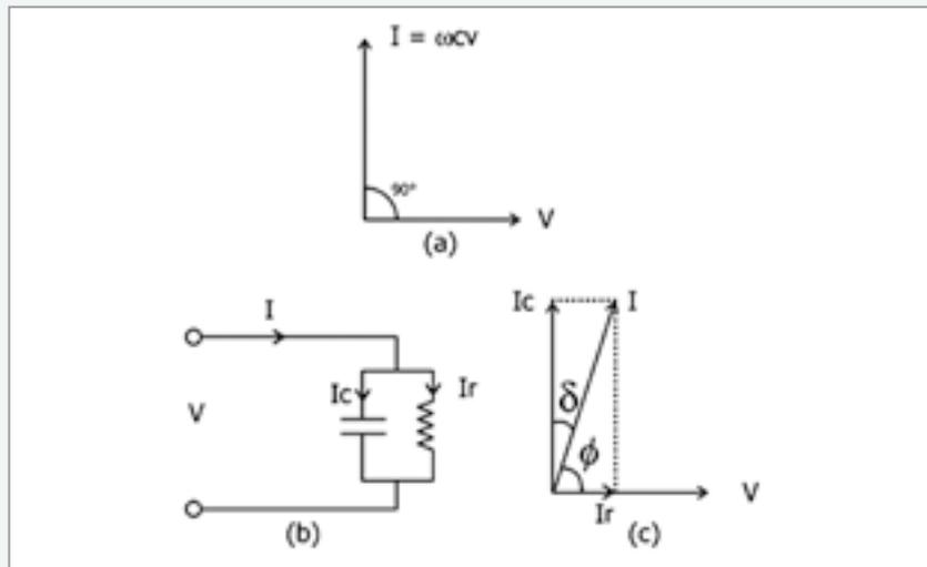
Figure 6. The loss angle  $\delta = 90 - \phi$  is the angle between the phasors  $I_c$  and  $I$
