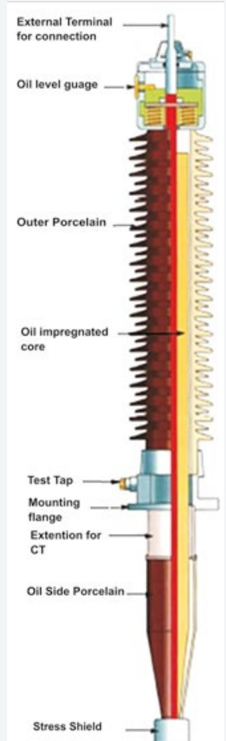
Figure 7a. Components of a condenser bushing [7]
