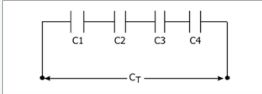
Figure 5. Equal capacitors in series
