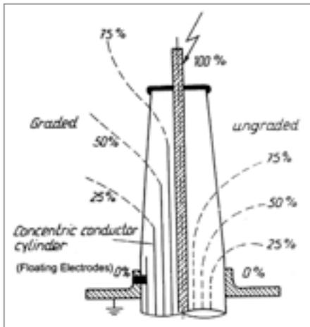
Figure 3. Comparison of potential distribution in graded and ungraded bushings [5]
