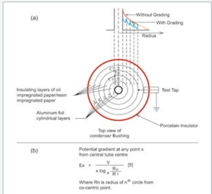
Figure 2. (a) The concept of potential graded condenser bushings [3]; (b) calculation of the potential gradient  $E_x$  at a distance  $x$  from the centre of the cylindrical tube/rod of the bushing [4]
