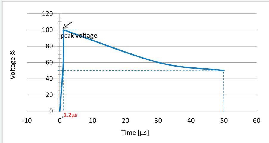
Figure 8. Lightning impulse voltage profile
