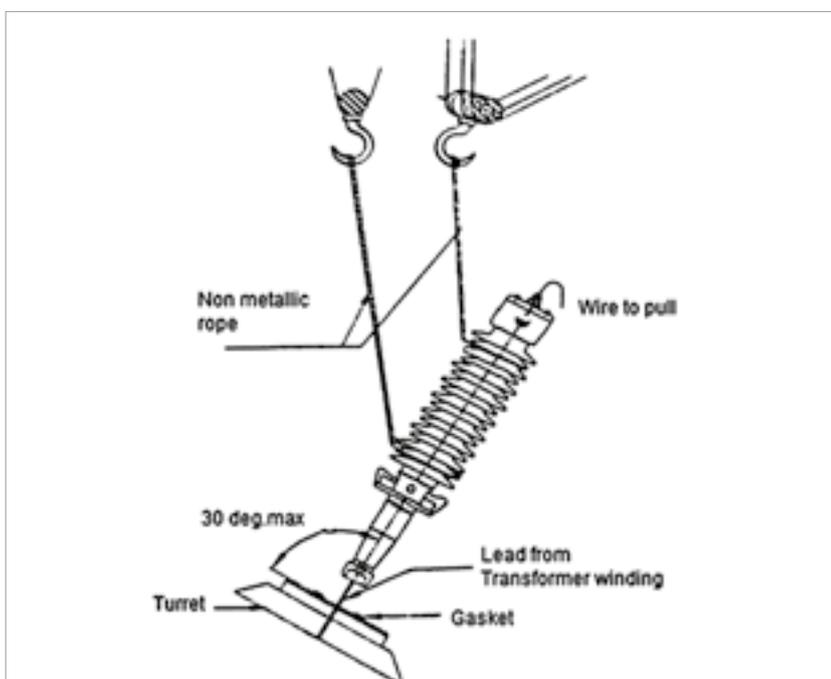
Figure 11. Installation/erection of a bushing (draw-lead type) [10]
