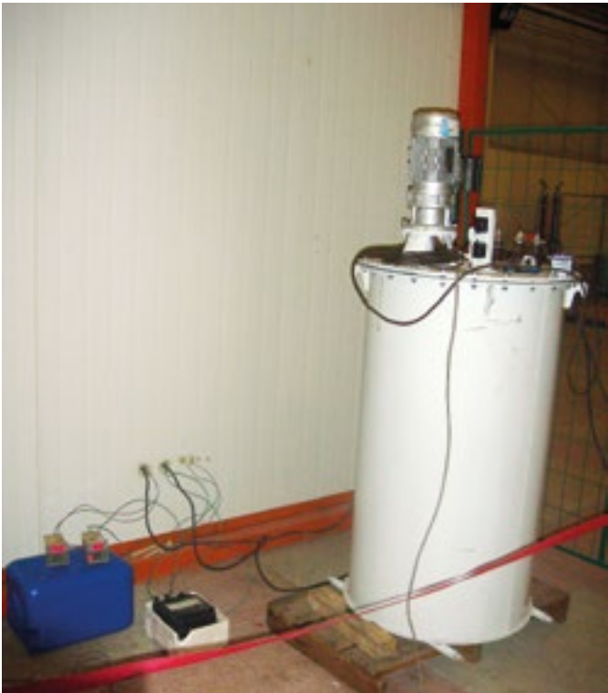
Figure 4. Low temperature test with current injection
