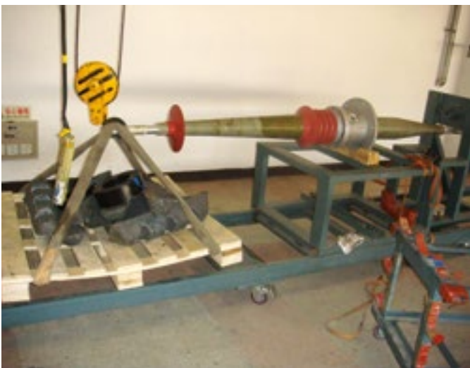
Figure 6. Heavy cantilever load test at 105 °C
