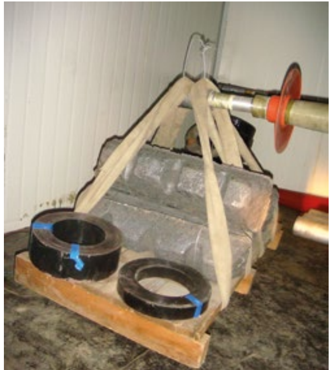
Figure 5. Cantilever load test at low temperature
