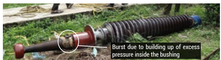
Figure 5b. The failed 245 kV, 1250 A, OIP bushing showing bursting of lower oil end insulator
