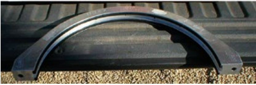
Figure 10. One half of a precision bolted aluminum clamp prior to mounting around a bushing
