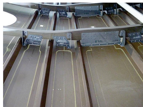
Figure 2 Integral skin-stringer structure of the fuselage
