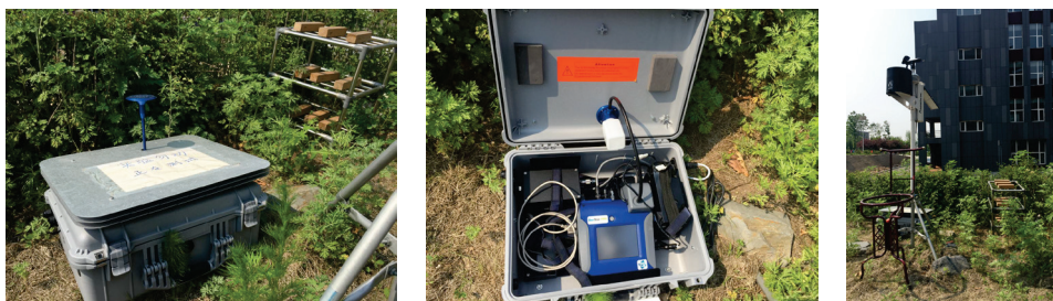
Figure 1 Experimental observation equipment (Left and middle: aerosol monitors; Right: weather station)
