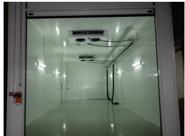
Figure 1 Insulated testing chamber
