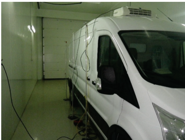
Figure 7 Arrangement of thermometers outside the insulated transport body
