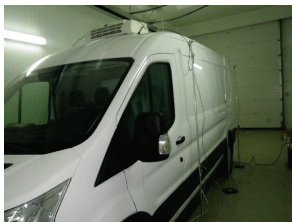
Figure 6 Arrangement of thermometers outside the insulated transport body
