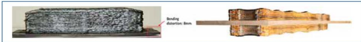
Slika 5. Deformacija kod WAAM komada (lijevo) i komad načinjen korištenjem Symmetrical Building strategije [3] Figure 5. Deformation on WAAM manufactured product (left) and product made using Symmetrical Building strategy [3]
