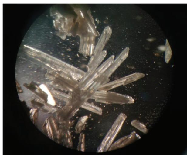
Fig. 2 – Microscopic observation of crystals of biocement from *Bacillus cereus* KLUVAA (4X magnification)
