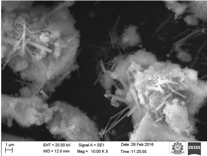
Fig. 4 – Characterization of bio cement using SEM
