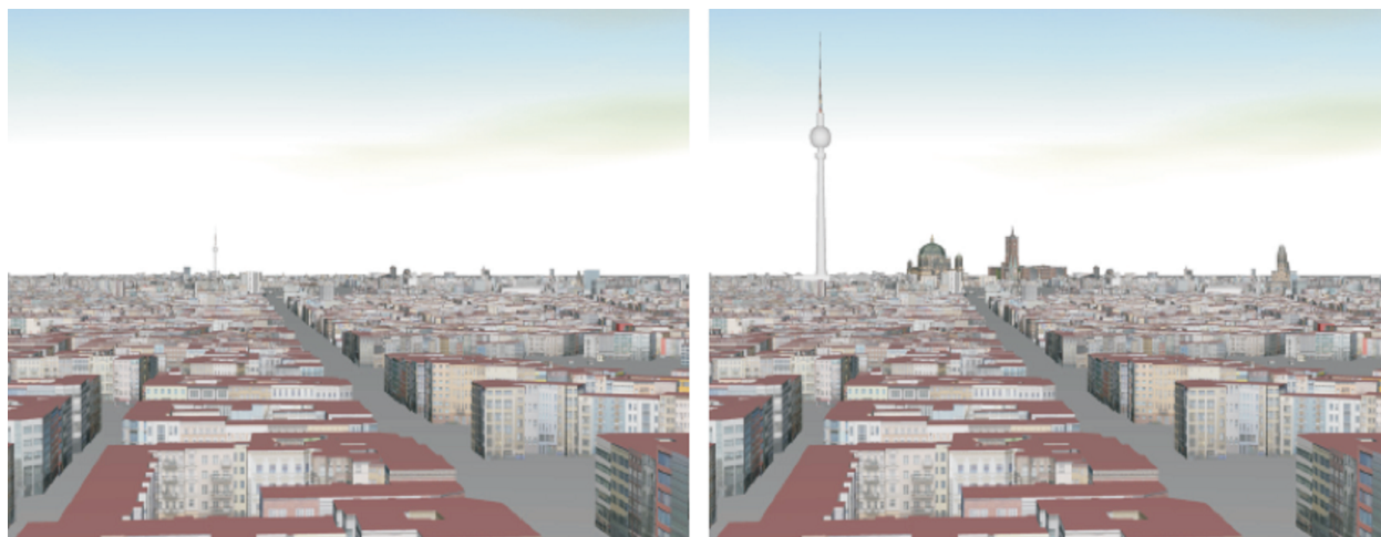
Fig. 2 A photorealistic 3D city model (left) and its non-photorealistic counterpart with visually accentuated landmarks (right) (Galander et al. 2007)
