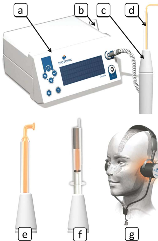
Figure 2. Ozonix generator used in this investigation: (a) generator; (b) patient grounding electrode; (c) applicator; (d) glass plasma electrode (for application in dentistry different shapes of electrodes are available, e.g. GI, AL, CA, PA probe); (e) investigated lens-shaped plasma electrode (GI probe, product number 1005, diameter = 8 mm) recommended for disinfection and stimulation of soft tissues; (f) ozone-producing syringe (KP probe) recommended for installation of gaseous ozone in treatment of root canals and periodontal pockets; (g) double plasma electrode (Omega probe) recommended for extra-oral treatment of pain and TMD (data according to manufacturer Biozonix GmbH, Munich, Germany – image created by Domagoj Prebeg).
