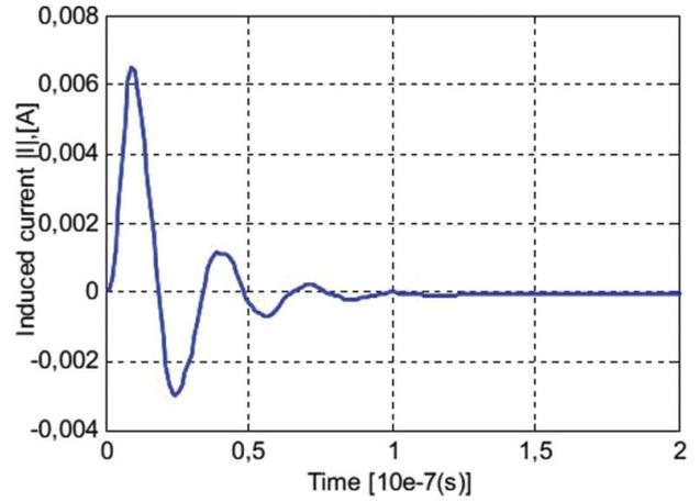
Figure 6. Transient current induced in the feet due to due to the bi-exponential pulse exposure.
