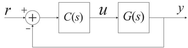
**Figure 1.** The unit negative feedback control structure.
