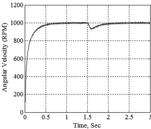
Figure 6. The load torque effect for Example 1.
