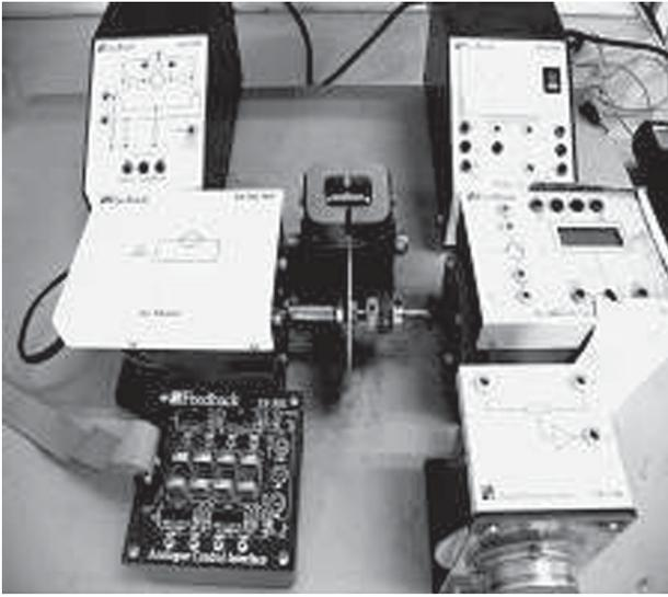
Figure 2. The DC servomotor plant in Example 1.
