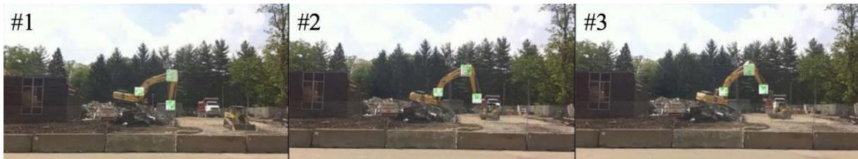
Figure 4. An example of tracking the arm (i.e. boom and stick) and bucket of an excavator (taken over and cropped up: Yuan *et al.*, 2016)
