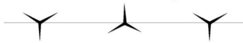
Figure 1 Positioning a tripod in relation to the leveling line (Tuno and Kogoj, 2012)
