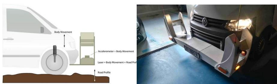
Figure 2. A view of the measurement vehicle Hawkeye 2000
