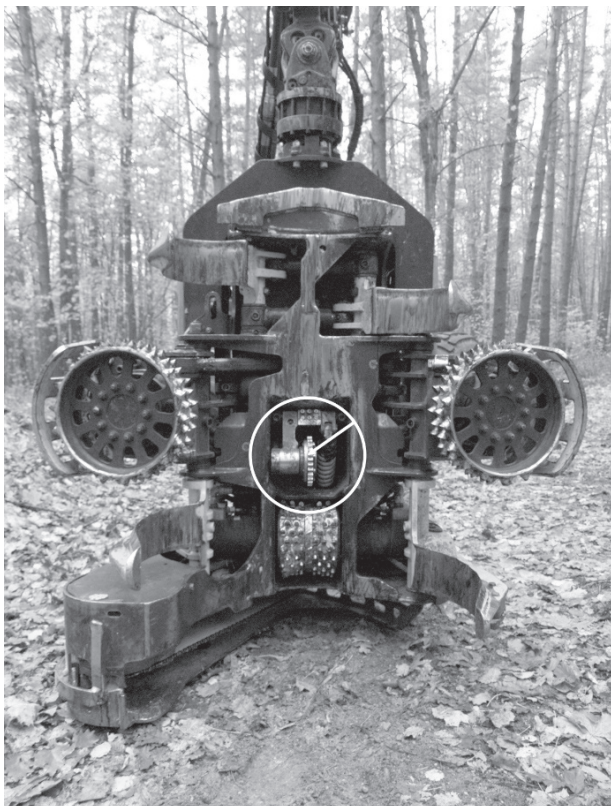
Fig. 1 Ponsse H7 harvester head (photo by Piotr S. Mederski) and measuring wheel (indicated with an arrow) in central part of head measure length of tree trunk by contact with its surface
