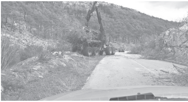
Fig. 1 Forwarder pulling out the fired Aleppo pine biomass from the fired forest
