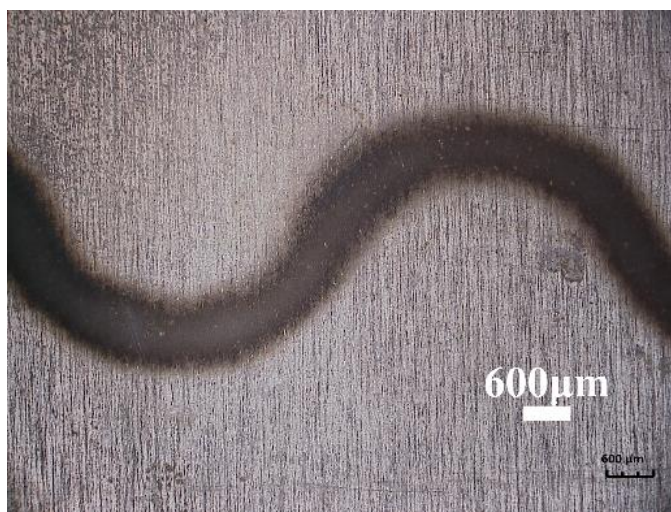
Figure 8. Electrochemical machining sample based on flexible cathode of EDTA-Cu and polyurethane
