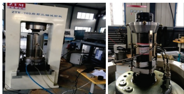
Figure 1 ZTR-203 electro-hydraulic servo rock three-axis test system
