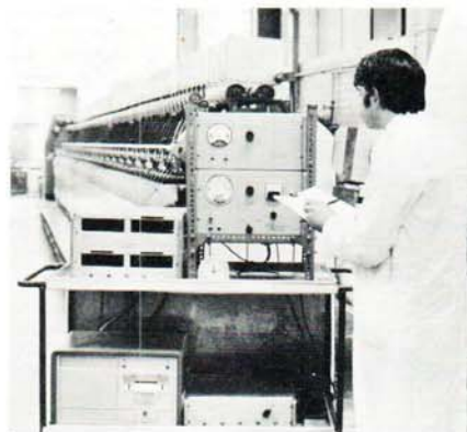
FIG. 6—Unit for assessment of dust levels in a major installation.
