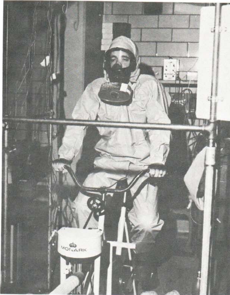
FIG. 3 - The vapor-barrier clothing (VBC) worn for the tests (except that this subject is not wearing the gloves or rubber boots).
