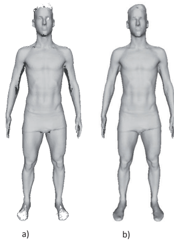
Figure 4. Point clouds of the digitalized human body: a) point cloud obtained by 3D scanning; b) point cloud prepared for 3D modelling
