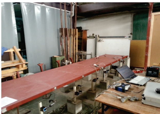
Figure 2 Grid bridge model during the test without additional mass
