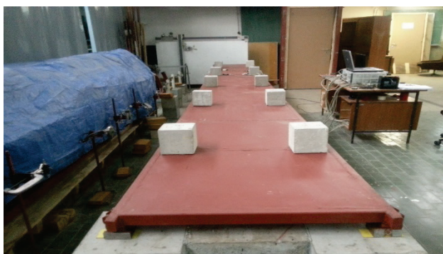
Figure 3 Grid bridge model during test with additional mass
