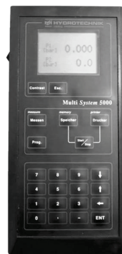
Figure 9 View of measuring equipment M5000 Hydrrotechnik
