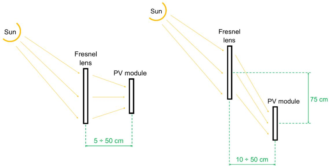
Figure 6. The tested configurations of Fresnel lens and PV module system
