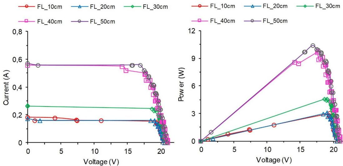
Figure 9. The I-V and P-V characteristics of PV module operating with Fresnel lens (which is placed above the PV module)
