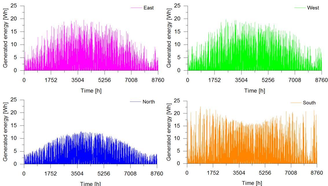
Figure 7. The estimated variations in electricity generation depending on the azimuth of considered PV module
