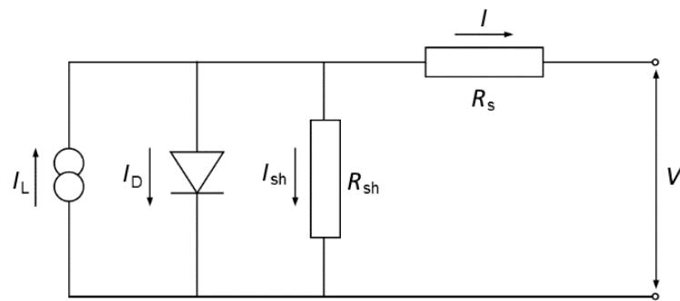
Figure 2. Equivalent electrical circuit of PV module
