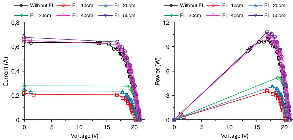
Figure 8. The I-V and P-V characteristics of PV module operating with Fresnel lens
