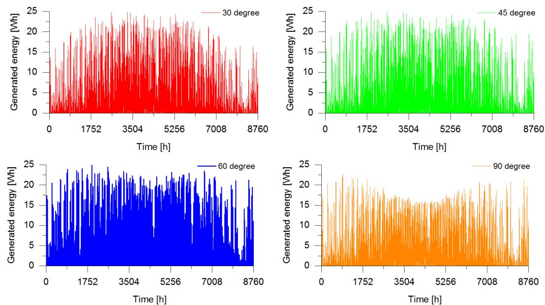
Figure 5. The estimated variations in electricity generation depending on the slope of considered PV module
