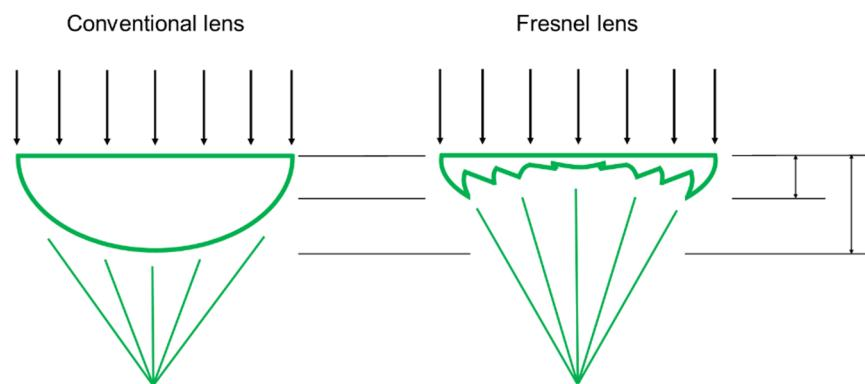
Figure 1. The comparison of conventional and Fresnel lens
