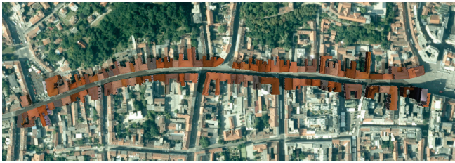
Figure 5 Roof textures assigned by the "random" method
