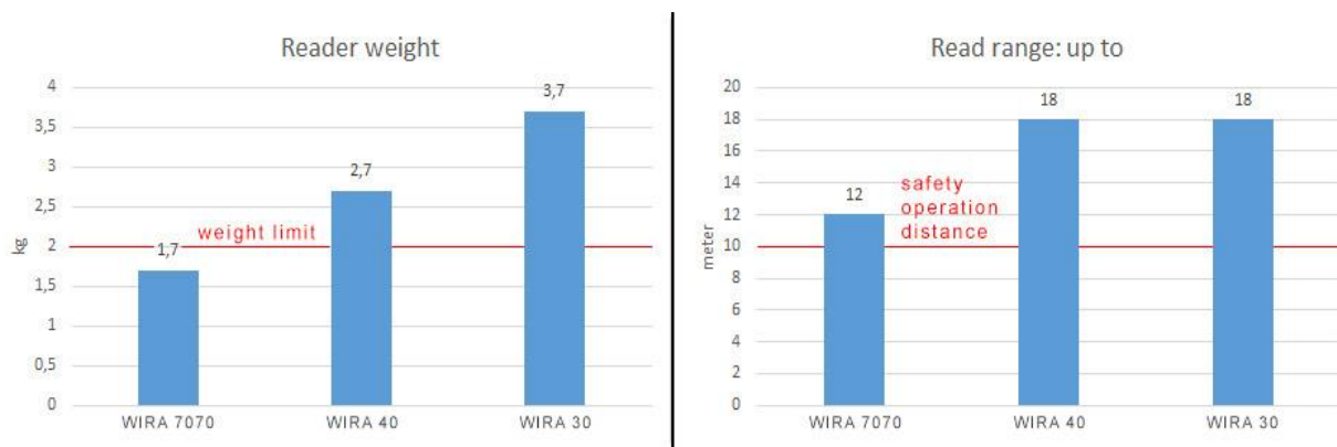
Figure 4. Parameter limits for selecting the RFID reader [15] (authors' edit of https://www.kathrein-solutions.com/datasheets ).
