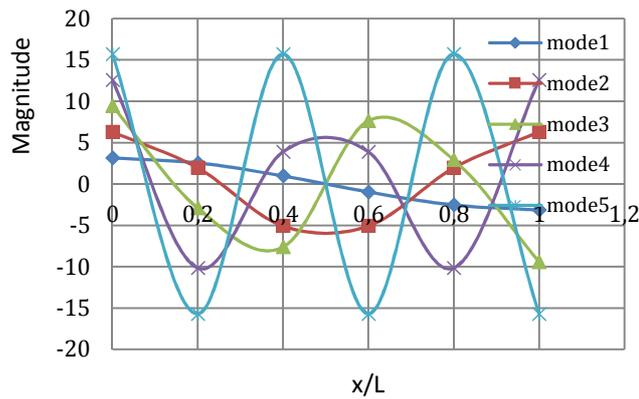
Fig. 5 Rotational vibration of the first five modes
