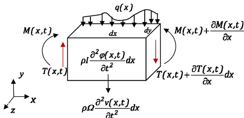
Fig. 2 Free-body diagram of an element of length dx
