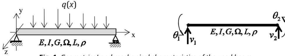
**Fig. 1** Geometrical and mechanical characteristics of the used beam
