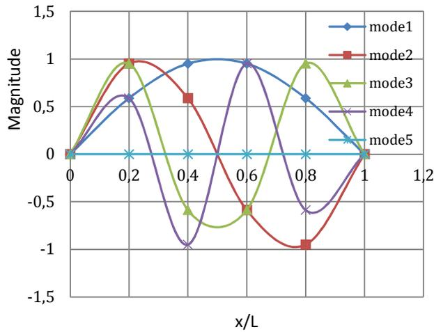
Fig. 4 Transversal vibration of the first five modes
