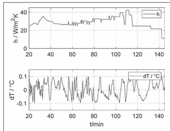
**Figure 1** Obtained  $h$  values along heating profile (upper) and  $dT$  for the obtained  $h$
