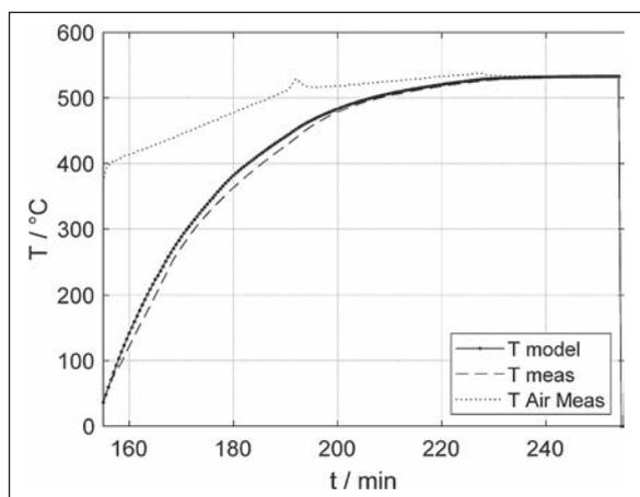
**Figure 3** Model prediction temperature profile and 4<sup>th</sup> measured profile together with furnace temperature, RMSE = 12,3 °C
