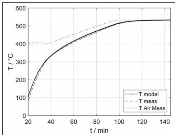
**Figure 2** Model prediction temperature profile and 3<sup>rd</sup> measured profile together with furnace temperature, RMSE = 10,1 °C
