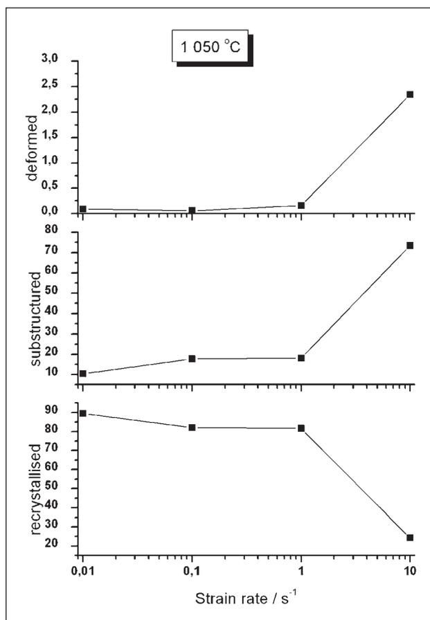
**Figure 5** The volume fractions of DRX grains at different strain rate
