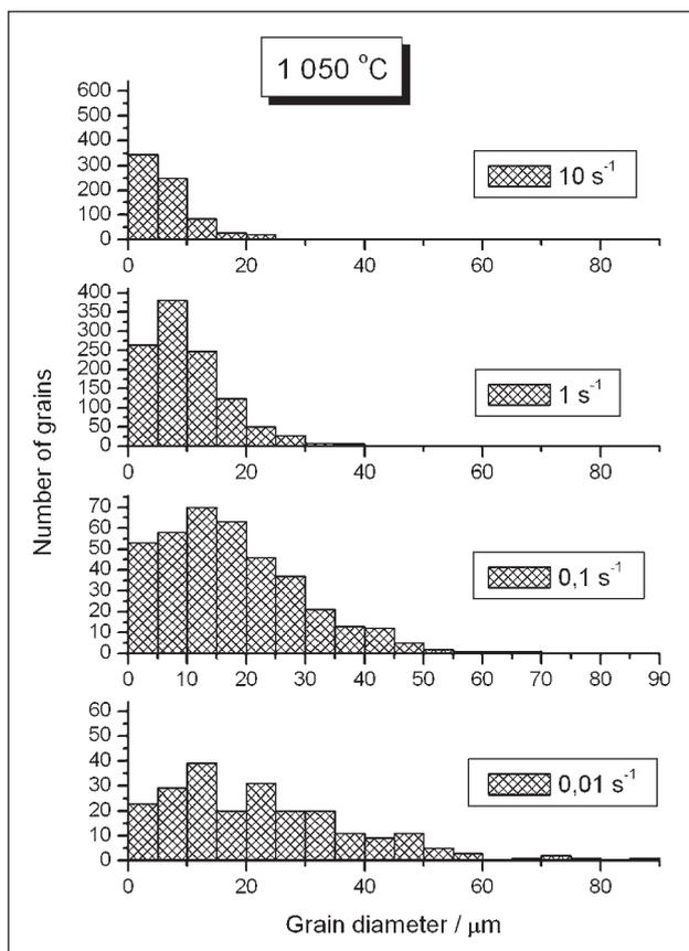
**Figure 4** Grain sizes distribution and number of grains of the alloy deformed at 1050 °C at different strain rates
