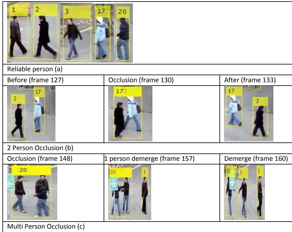
Fig. 10. Tracking result on PETS2009-S2L1. First rows (a) refer to PETS2009-S2L1 reliable persons, whose features are stored, whereas the last row refers to two person occlusion (b) as well as multi person occlusion (c) of same sequence.
