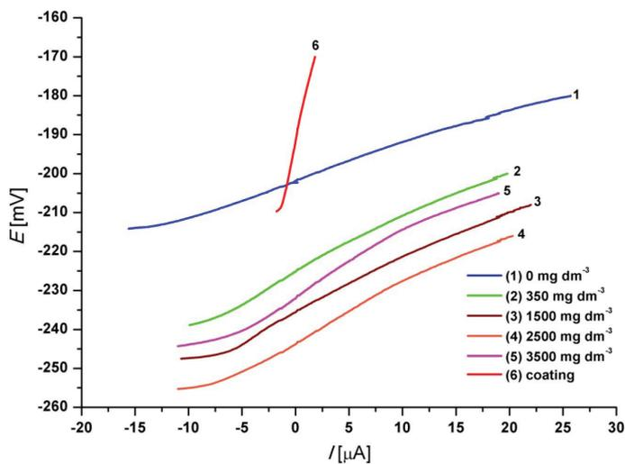
Fig. 2 – Linear polarization curves for copper in  $0.51 \text{ mol dm}^{-3}$  NaCl solution without stirring as a function of various propolis extract concentrations
