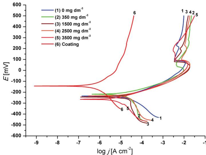
Fig. 3 – Potentiodynamic polarization curves in  $0.51 \text{ mol dm}^{-3}$  NaCl solution as a function of various propolis extract concentrations
