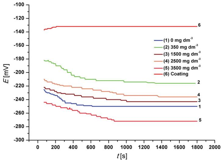
Fig. 1 – Dependence of corrosion potential for Cu in  $0.51 \text{ mol dm}^{-3}$  NaCl solution in the absence and presence of propolis extract as a function of time
