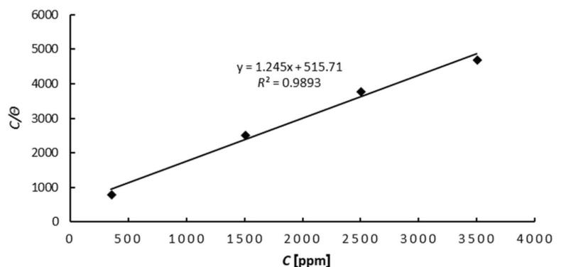
Fig. 4 – Langmuir's adsorption isotherm for propolis adsorption process on the copper surface in NaCl solution
