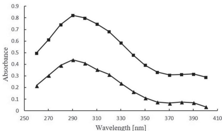
Fig. 6 – UV-Visible spectra of test solution with propolis extract ( $3500 \text{ mg dm}^{-3}$ ): before immersion ( $\blacksquare$ ), and after 48 hours immersion ( $\blacktriangle$ ) of copper samples in solution
