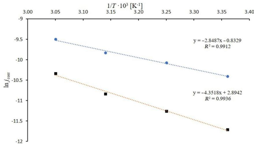
Fig. 5 – Arrhenius's plots for Cu in  $0.51 \text{ mol dm}^{-3}$  NaCl: in the absence ( $\bullet$ ), and in presence of propolis extract ( $\blacksquare$ ) in concentration of  $3500 \text{ mg dm}^{-3}$
