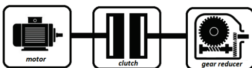
Figure 1 Electromechanical module – exemplary structural scheme
