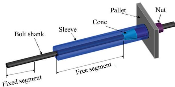
Figure 2 Structure of the CRLD bolt
