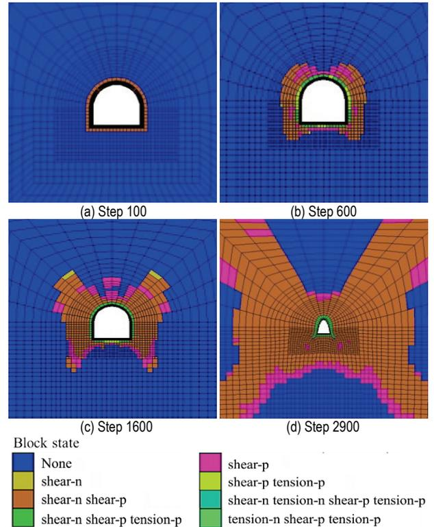
Figure 6 Distribution of the plastic zone under the high pretension bolt support
