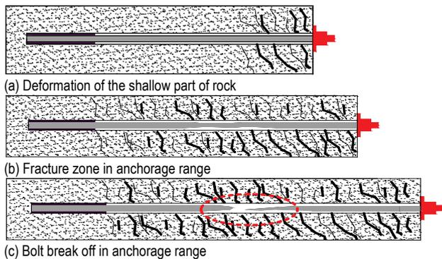
Figure 13 Failure stages of high pretension bolt
