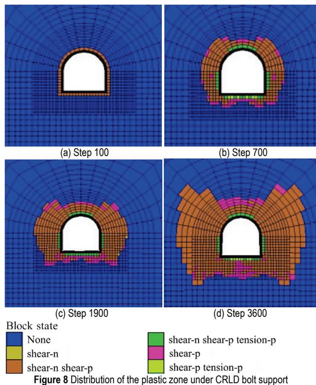
Figure 8 Distribution of the plastic zone under CRLD bolt support
