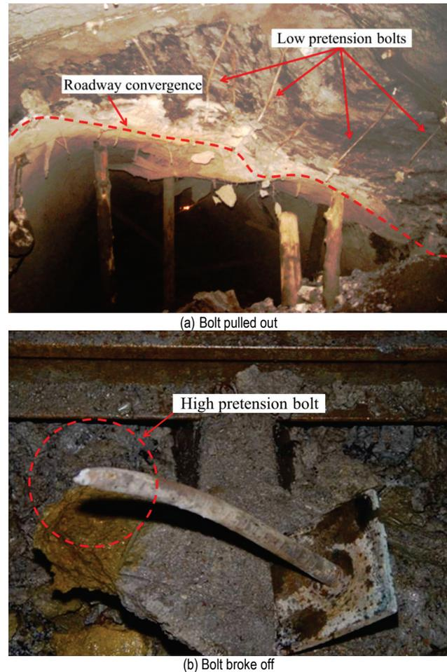
Figure 1 Failure of bolts in Nanshan Coal Mine
