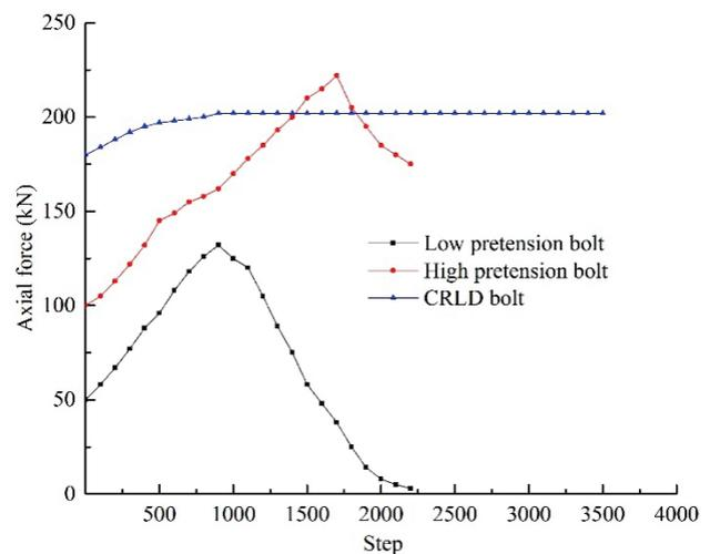
Figure 10 Monitoring curves of the axial force for different bolts
