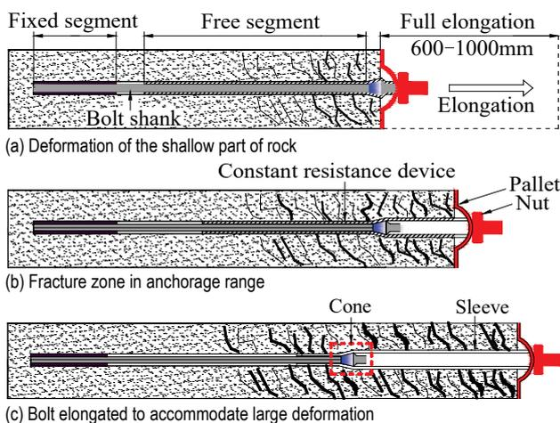
Figure 14 Working principle of CRLD bolt
