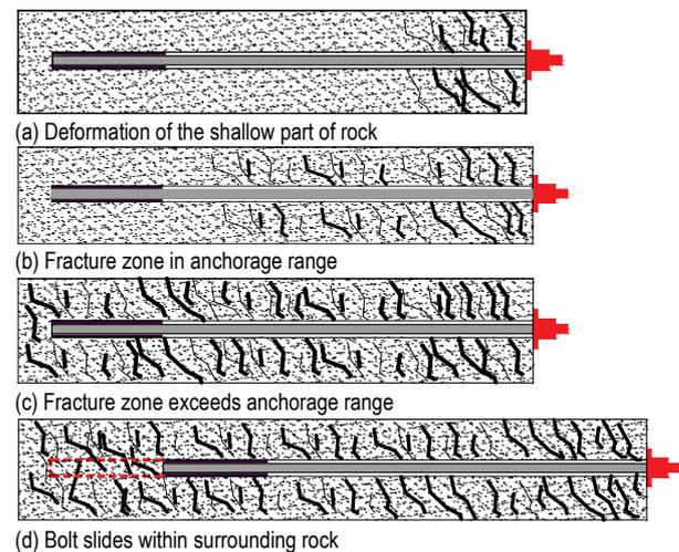
Figure 12 Failure stages of low pretension bolt
