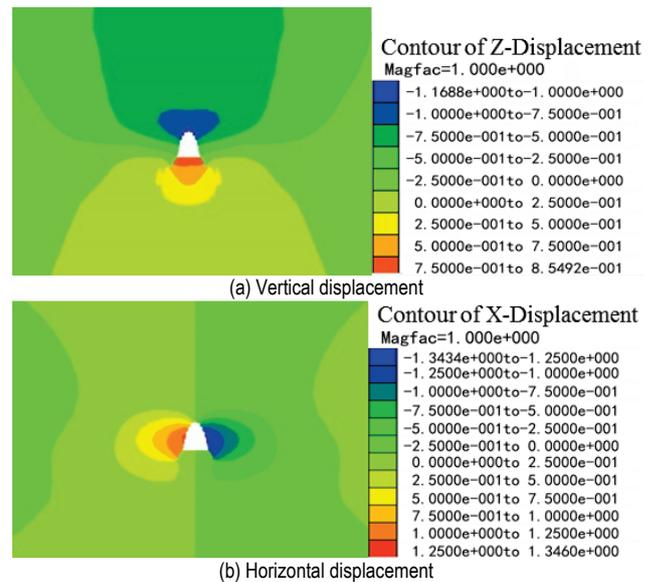
Figure 7 Deformation of the roadway under high pretension bolt support
