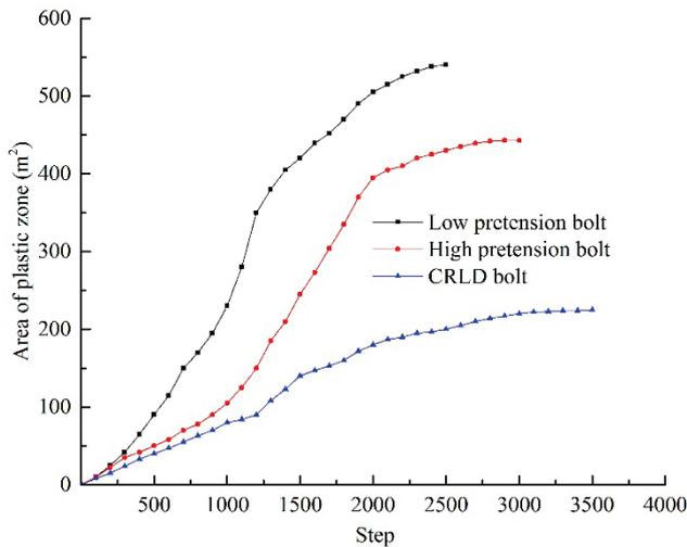
Figure 11 Curves of plastic zone areas under different bolts support
