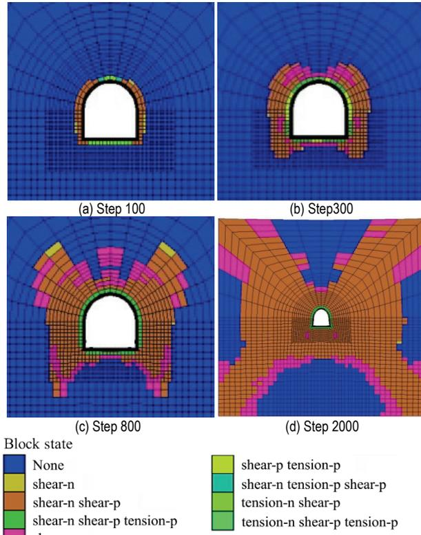
Figure 4 Distribution of the plastic zone under the low pretension bolt support
