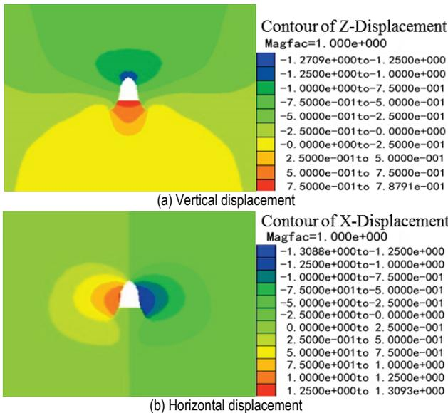
Figure 5 Deformation of the roadway under the low pretension bolt support
