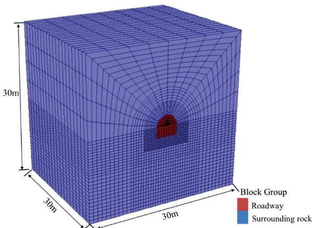
Figure 3 Schematic diagram of the global model
