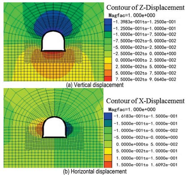
Figure 9 Deformation of the roadway under CRLD bolt support
