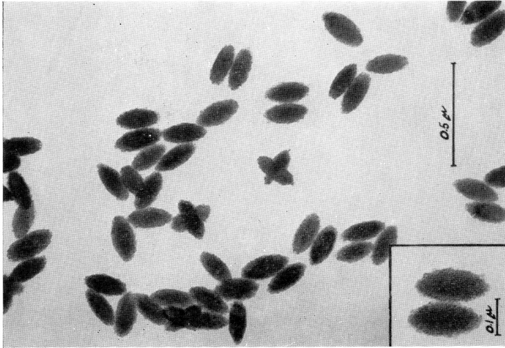
(a) Electron micrograph of unsectioned barium sulfate particles (System S-45) formed 10 minutes after the starting of the reaction. Magnification: 60,000 : 1. Detail shows particles at magnification 100,000 : 1.
