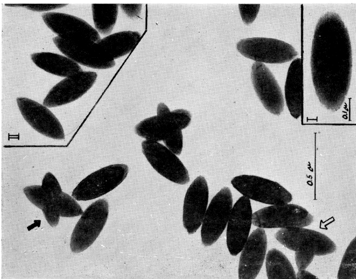
Fig. 2. Electron micrograph of unsectioned barium sulfate particles (System S-58) formed 45 minutes after the starting of the reaction. Magnification: 60,000 : 1. Detail I shows a particle at magnification 100,000 : 1. Detail II shows three overlapped particles
