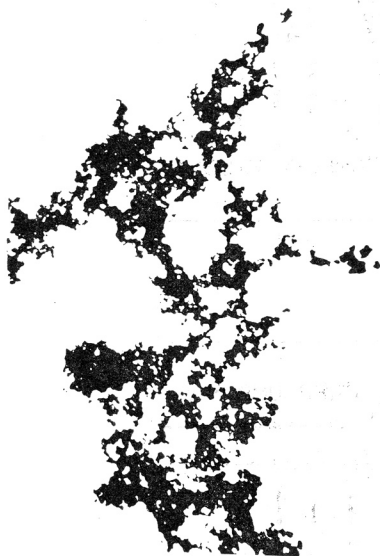
a) Electron micrograph of thorium hydroxide formed at pH = 4.48 is represented. The concentration of the reactants is 1.25 mM thorium nitrate, 100 mM sodium fumarate and 10 mM nitric acid.
