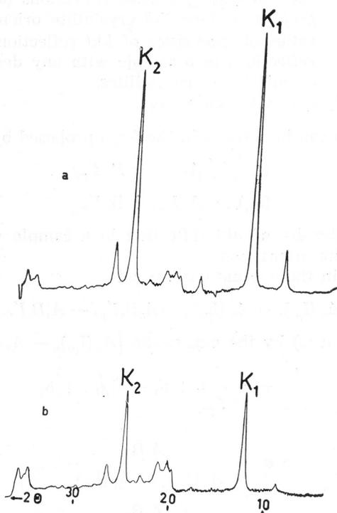
Fig. 1. X-ray pattern of kaolinite; a) high degree and b) low degree of preferential crystallite orientation.  $K_1$  corresponds to  $001$  reflection,  $K_2$  corresponds to  $002$  reflection.
