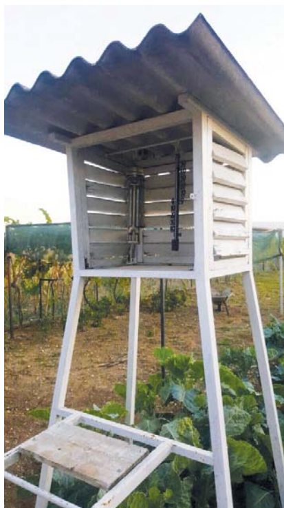
Fig. 1. Meteorological shelter of the measuring station in Vitina
